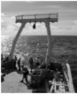
Part of the working deck with the A-frame at the stern of the Australian research vessel Franklin , seen during the deployment of a surface buoy for meteorological and oceanographic measurements.
